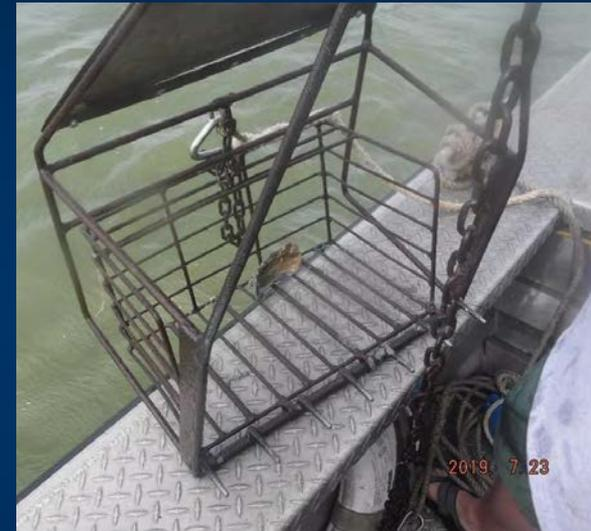
Frame: constructed with 13 mm diameter cold rolled steel rod 495 mm wide x 241 mm high x 1,000 mm long.
